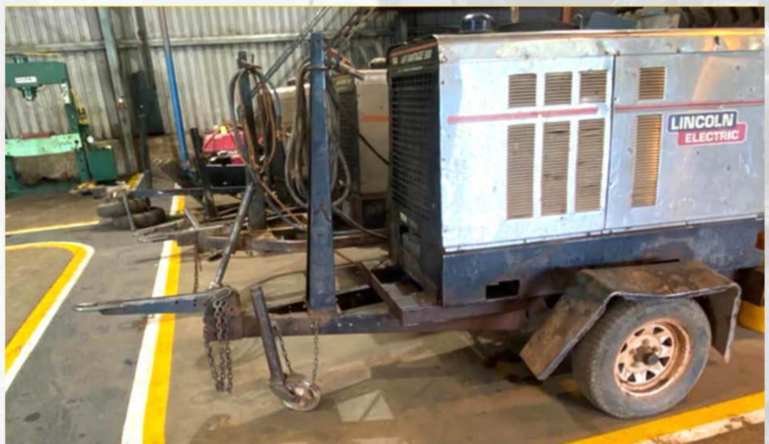
MOBILE WELDERS - LINCOLN AIR VANTAGE 500 WELDING MACHINES.
