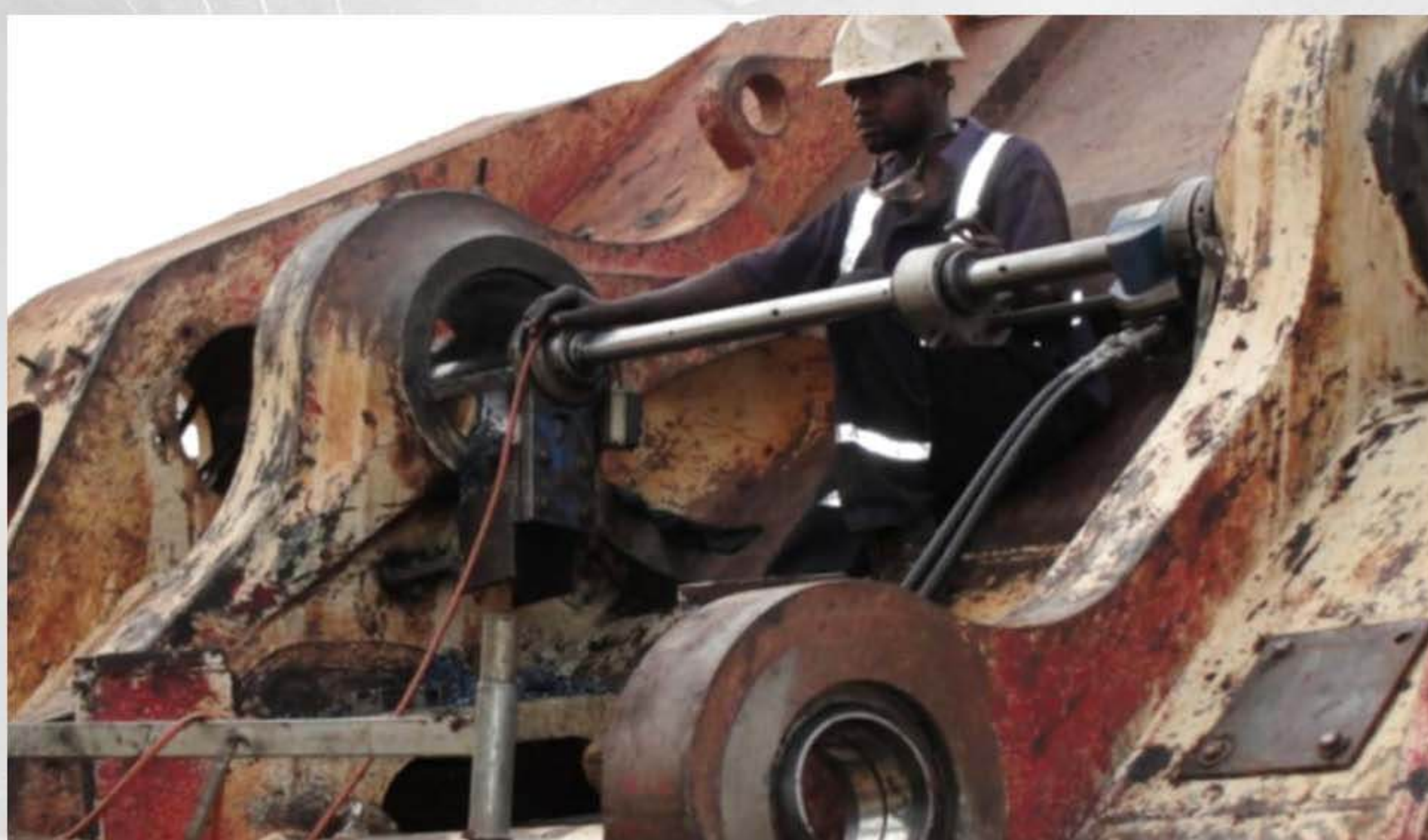
LINE BORING IN THE MINE ON AN RH170 EXCAVATOR BUCKET.
