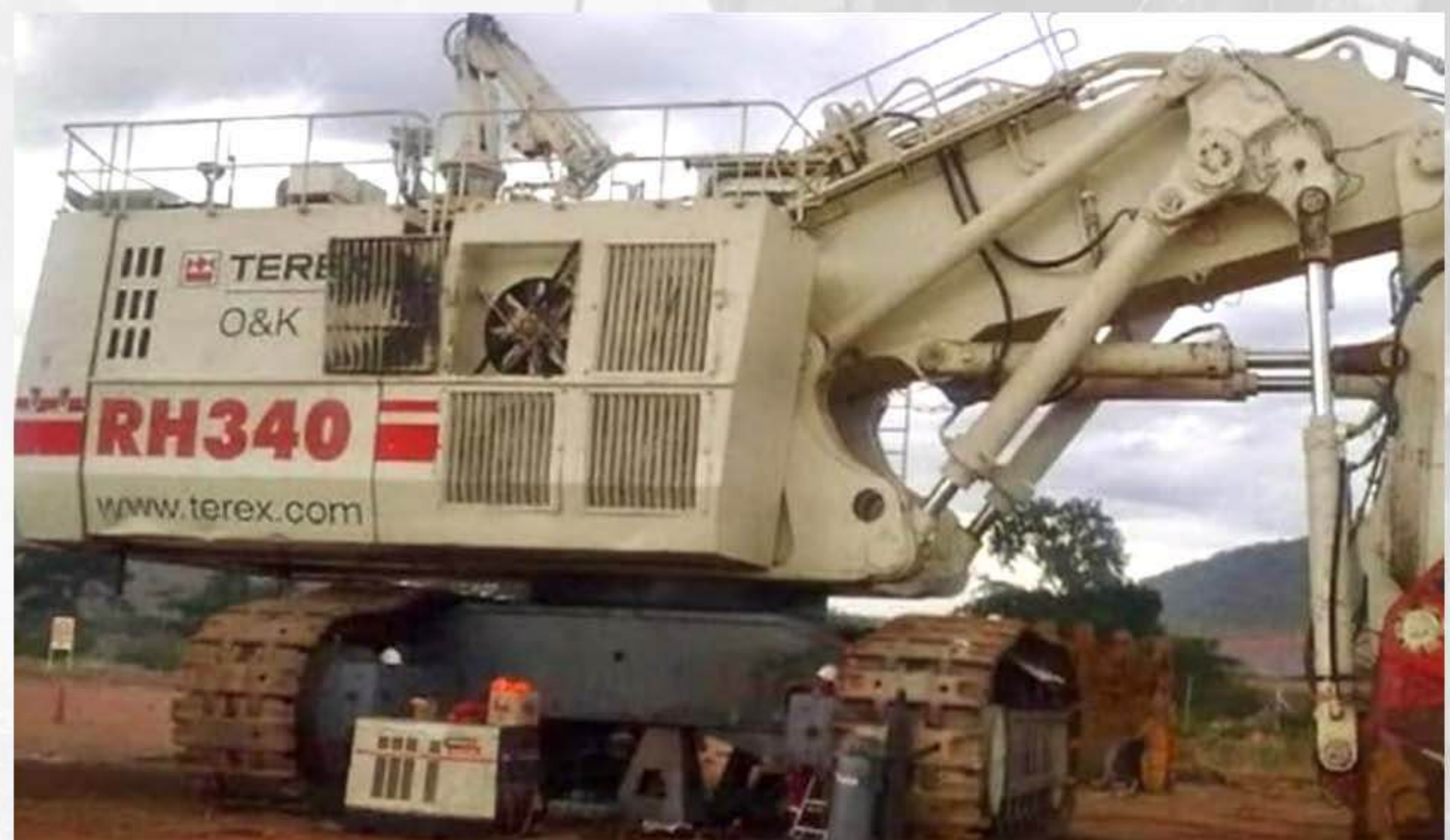
RH340 UNDERCARRIAGE REBUILD ON GOING AT GEITA GOLD MINING.
