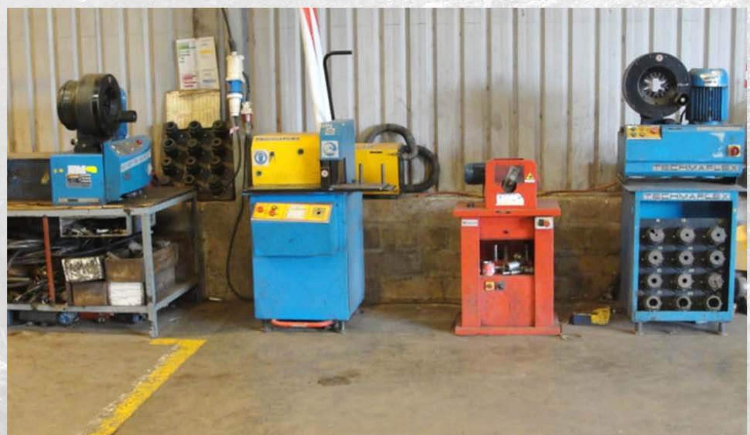
HYDRAULICS HOSE ASSEMBLY SECTION - EQUIPMENT SET UP
