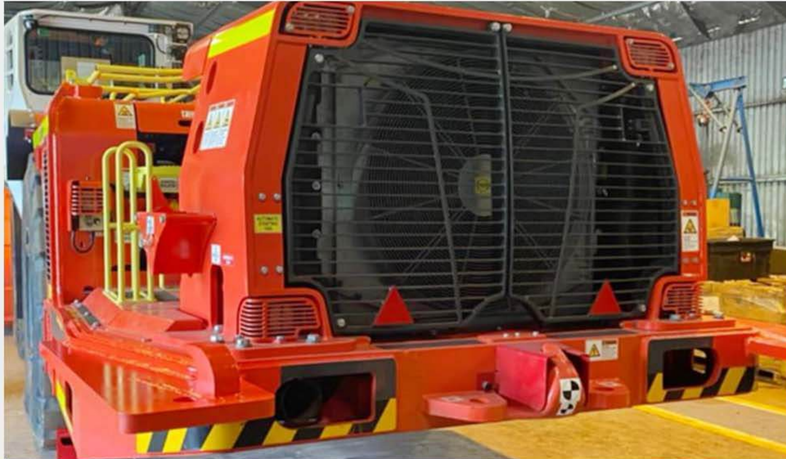
SANDVIK LOADER BACK VIEW OF WELDED DEFLECTOR PLATE ON BOTH ENDS.
